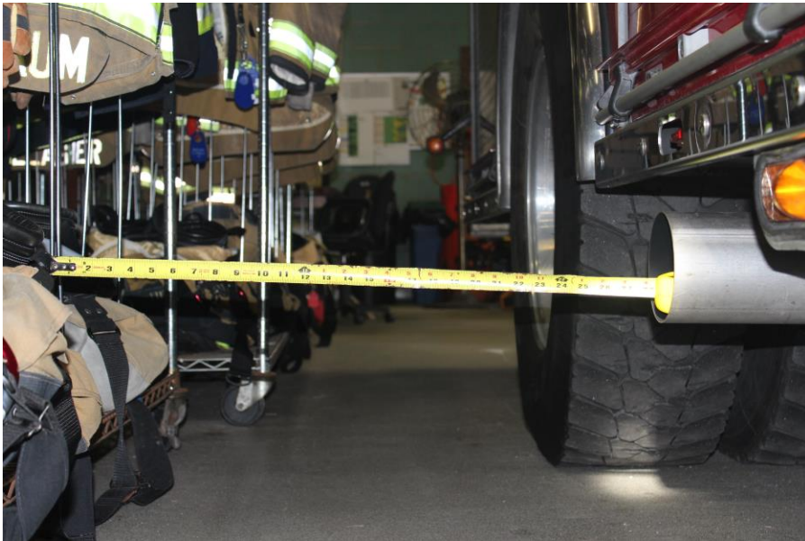
Diesel exhaust is released within 2' of where Firefighters don their turnout gear
